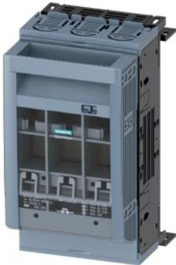
SENTRON, Fuse switch disconnector 3NP1, 3-pole, NH00, 160 A, for Busbar system 8US 60 mm, Box terminal, Cover level 32/70 mm
