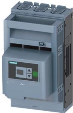
SENTRON, Fuse switch disconnector 3NP1, 3-pole, NH00, 160 A, for assembly and installation on mounting plate, Box terminal, Fuse monitoring: electronic EFM20, Cover level 45 mm
