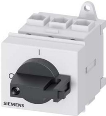
SENTRON, Switch disconnector 3LD, main switch, 3-pole, I<sub>u</sub>: 25 A, Operating power / at AC-23 A at 400 V: 9.5 kW, installation in distribution boards, knob-operated mechanism, black, handle direct at the switch
