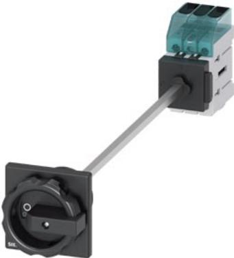
Load disconnector 3LD3, I<sub>u</sub> 40 A Main switch 3-pole Rated operating capacity at AC-23 A at 400 V 18.5 kW floor mounting Basic switch with door coupling Central hole mounting 22.5mm Rotating drive black 66 x 66 mm
