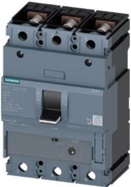
circuit breaker 3VA1 IEC Frame 250 breaking capacity class H Icu=70 kA @ 415 V 3-pole, starter protection TM120M, AM, In=200 A without overload protection short-circuit protection li=6...14 x In nut keeper kit
