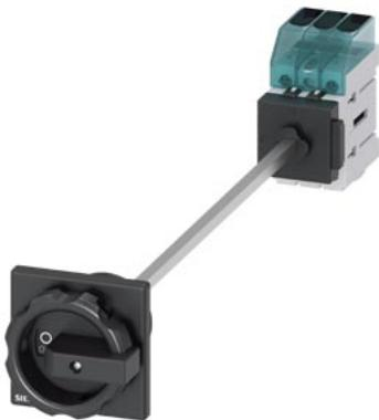
Load disconnector 3LD3, Iu 63 A Main switch 3-pole Rated operating capacity at AC-23 A at 400V 22.0 kW floor mounting Basic switch with door coupling Central hole mounting 22.5mm Rotating drive black 66 x 66 mm
