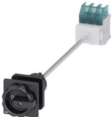
SENTRON, Switch disconnector 3LD, main switch, 3-pole, I<sub>u</sub>: 32 A, Operating power / at AC-23 A at 400 V: 11.5 kW, floor mounting with door coupling, rotary operating mechanism, black, central mounting 22.5 mm of the handle
