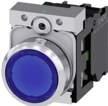
Illuminated pushbutton, 22 mm, round, metal, shiny, blue, pushbutton, flat, momentary contact type, with holder, 1 NO, LED module with integrated LED 24 V AC/DC, screw terminal
