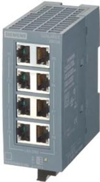
SCALANCE XB008 unmanaged Industrial Ethernet Switch for 10/100 Mbit/s; for setting up small star and line topologies; LED diagnostics, IP20, 24 V DC power supply, with 8x 10/100 Mbit/s Twisted Pair ports with RJ45 sockets; Manual available as a download
