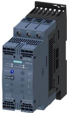
SIRIUS soft starter S2 63 A, 37 kW/500 V, 40 °C 400-600 V AC, 24 V AC/DC spring-type terminals
