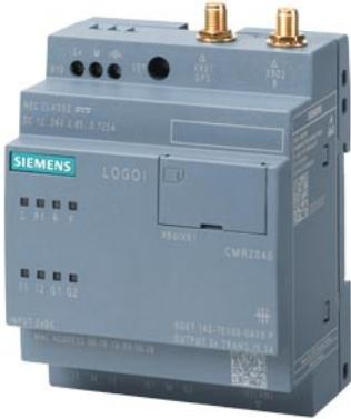
LOGO! CMR2040 communication module for connection LOGO! 8 to LTE network; 1 RJ45 port for Ind. Ethernet connection to LOGO! 8; 2xDI; 2xDO; write/read access to LOGO! variables; SMS dispatch/ receiving of text messages; email dispatch; position detection GPS; time synchronization/ forwarding with real time clock; Configuration/diagnostics via web interface; Remote access via OpenVPN/HTTPs, DynDNS, observe national approval! Manual available as a download .
