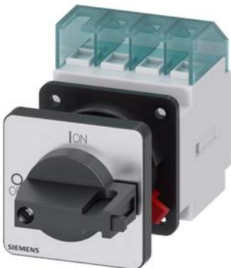
SENTRON, Switch disconnector 3LD, main switch, 3-pole, Iu: 16 A, Operating power / at AC-23 A at 400 V: 7.5 kW, front-mounted, knob-operated mechanism, black, central mounting 22.5 mm of the handle
