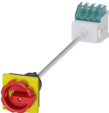
SENTRON, Switch disconnector 3LD, emergency switching-off switch, 3- pole, Iu: 16 A, operating power / at AC-23 A 400 V: 7.5 kW, floor mounting with door coupling, rotary operating mechanism, Red / yellow, 4-hole mounting of the handle
