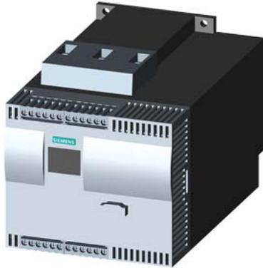
SIRIUS soft starter Values at 400 V, 40 °C standard: 77 A, 37 kW Inside-delta: 133 A, 75 kW 200-460 V AC, 230 V AC Screw terminals !!! Phased-out product !!! Successor is SIRIUS 3RW5, Preferred successor type is >>3RW5526-1HA14<<
