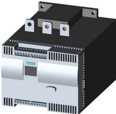
SIRIUS soft starter Values at 400 V, 40 °C standard: 250 A, 132 kW Inside-delta: 433 A, 250 kW 200-460 V AC, 230 V AC Screw terminals !!! Phased-out product !!! Successor is SIRIUS 3RW5, Preferred successor type is >>3RW5544-6HA14<<
