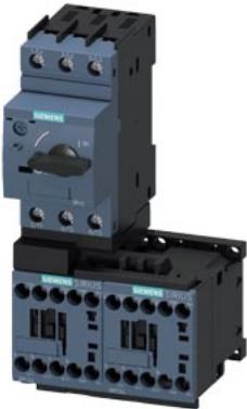
Load feeder fuseless, Reversing duty 400 V AC, Size S00 1.10...1.60 A 24 V DC screw terminal for installation on standard mounting rail (also fulfills type of coordination 1) Type of coordination 2,  $I_q = 150 \text{ kA}$  1 NC (contactor)
