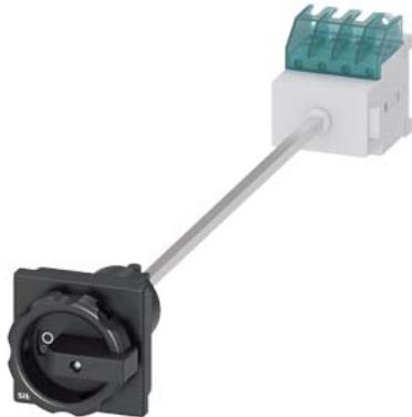
SENTRON, Switch disconnector 3LD, main switch, 4-pole, I<sub>u</sub>: 16 A, Operating power / at AC-23 A at 400 V: 7.5 kW, floor mounting with door coupling, rotary operating mechanism, black, 4-hole mounting of the handle
