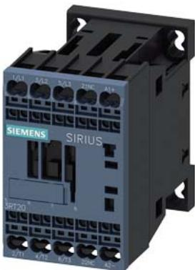
power contactor, AC-3e/AC-3, 16 A, 7.5 kW / 400 V, 3-pole, 24 V DC, auxiliary contacts: 1 NC, spring-loaded terminal, size: S00
