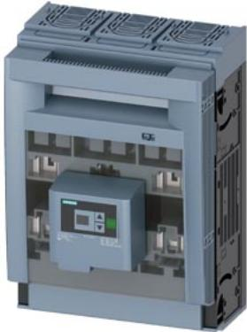
SENTRON, Fuse switch disconnector 3NP1, 3-pole, NH2, 400 A, for assembly and installation on mounting plate, flat terminal, Fuse monitoring: electronic EFM20, Cover level 70 mm
