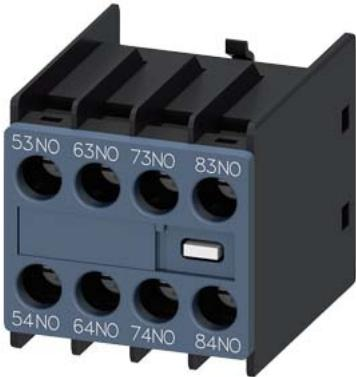
auxiliary switch, on the front, 4 NO, 53/54, 63/64, 73/74, 83/84, current path: 1 NO, 1 NO, 1 NO, 1 NO, screw terminal, physically coded, only with contactor relays 3RH2140 and 3RH2440 combinable (according to EN 50011)
