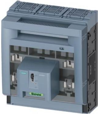
SENTRON, Fuse switch disconnector 3NP1, 3-pole, NH3, 630 A, for assembly and installation on mounting plate, flat terminal, Fuse monitoring: electromechanical, Cover level 70 mm
