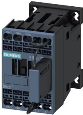
contactor relay railway, 2 NO + 1 NC, 24 V DC, 0.7-1.25\* Us, with integrated suppressor diode, spring-loaded terminal, frame size S00
