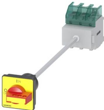
SENTRON, switch disconnector 3LD, EMERGENCY OFF switch, 3-pole,  $I_u$ : 63 A, Operating power / at AC-23 A at 400 V: 22 kW, floor mounting with door coupling, defeatable knob-operated mechanism, red/yellow, 4-hole mounting of the handle
