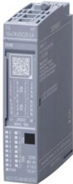
SIMATIC ET 200SP, digital output module, DQ 16x 24 V DC/0.5 A high feature, source output PNP, switching to P potential, packing unit: 1 unit, suitable for BU type A0, color code CC00, channel diagnostics for: short-circuit and wire break, supply voltage, channel fault LED
