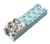
SIMATIC DP, Basic module BM 143 ET 200ECO: 8 DI/8 DO, 1.3A, 8xM12, Duplicate assignment, IP65/67, Connection block 6ES7194-3AA00-0.A0 order separately
