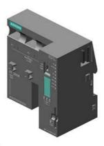
SIMATIC DP, IM151-8 PN/DP CPU f. ET200S, 192 KB work memory, int. PROFINET interface (with three RJ45 ports) as IO controller, without battery MMC required
