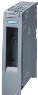
SIMATIC ET 200MP, multi-fieldbus, interface module IM 155-5 MF HF, IM 155-5 MF HF, EtherNet/IP and Modbus TCP, 2 flexible ports via plug-in SIMATIC BusAdapter (sold separately), max. 30 I/O modules, multi-hot-swap with active backplane (sold separately), IRT with 250 µs, shared device with 4 controllers (1440 bytes each), 256 bytes per I/O module, MRP, MRPD, S2 redundancy, PN security class 1, optional cable grip (sold separately) PN security class 1, optional cable grip (sold separately)
