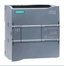
\*\*\*Spare part\*\*\* SIMATIC S7-1200, CPU 1212C, compact CPU, AC/DC/relay, onboard I/O: 8 DI 24 V DC; 6 DO relay 2 A; 2 AI 0-10 V DC, Power supply: AC 85-264 V AC at 47-63 Hz, Program/data memory 25 KB
