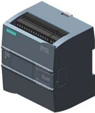
SIMATIC S7-1200, CPU 1212C, compact CPU, AC/DC/relay, onboard I/O: 8 DI 24 V DC; 6 DO relay 2 A; 2 AI 0-10 V DC, Power supply: AC 85-264 V AC at 47-63 Hz, Program/data memory 50 KB
