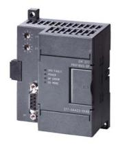
$^{***}$  spare part  $^{***}$  SIMATIC S7-200, PROFIBUS DP Slave module, 9.6 KB to 12 MB, 1 interface PROFIBUS-DP/MPI
