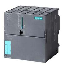
\*\*\*Spare part\*\*\* SIMATIC S7-300 CPU 319-3 PN/DP, Central processing unit with 1.4MB memory, 1st interface MPI/DP 12 Mbit/s, 2nd interface DP master/slave 3rd interface Ethernet PROFINET, Micro Memory Card required
