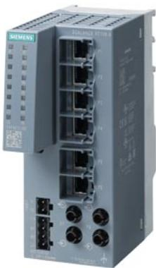
SCALANCE XC106-2, Unmanaged IE switch, 6x 10/100 Mbit/s RJ45 ports, 2x 100 Mbit/s Multimode BFOC, LED diagnostics, error-signaling contact with set pushbutton, redundant power supply Manual available as a download .
