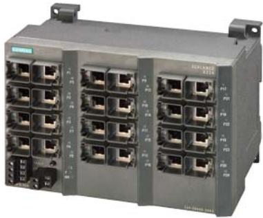
SCALANCE X224, managed IE switch, 24x 10/100 Mbit/s RJ45 ports, LED diagnostics, error-signaling contact with set pushbutton, redundant power supply, PROFINET IO device, network management, can be operated in red. ring, including electronic manual on CD-ROM, C-PLUG optional.
