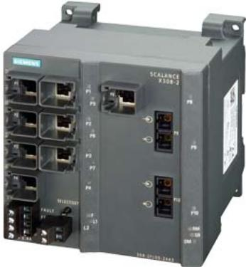
\*\*\*\*\* spare part \*\*\*\*\* SCALANCE X308-2, managed plus IE switch, 2x 1000 Mbit/s MM SC 1x 10/100/1000 Mbit/s and 7x 10/100 Mbit/s RJ45 ports, LED diagnostics, error signaling contact with select/set pushbutton, PROFINET IO device, network management, integrated redundancy manager, office features (RSTP, VLAN, IGMP,..) C-PLUG in scope of delivery 30.
