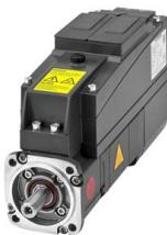
SINAMICS SERVO-DRIVE DISTRIBUÍDO S120M AH36, M(0)=1,00Nm n(N)=3000 RPM, ENTRADA: DC 600V ABSOLUTE ENCODER 20 BIT NATURAL AIR COOLING, IM B5, IM V1, IM V3 GRAU DE PROTEÇÃO: EIXO IP65 COM TOLERÂNCIA DE CHAVE INSTALADA N; COM FREIO DE RETENÇÃO
