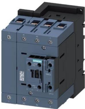
power contactor, AC-3, 65 A, 30 kW / 400 V, 4-pole, 175-280 V AC/DC, 50/60 Hz, with integrated varistor, main contacts: 2 NO + 2 NC, auxiliary contacts: 1 NO + 1 NC, screw terminal, size: S3
