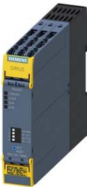
SIRIUS safety relay Basic unit Advanced series 3 electronic enabling circuits 1 electronic signaling circuit  $U_s = 24$  V DC screw terminal
