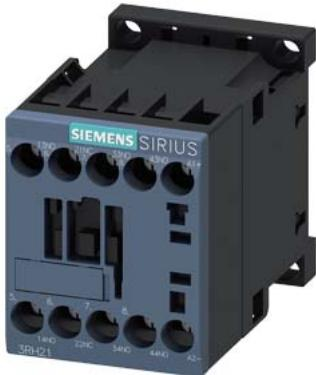
coupling contactor relay, 3 NO + 1 NC, 24 V DC, 0.7-1.25\* Us, screw terminal, frame size S00, suitable for PLC outputs, not expandable with auxiliary switch expandable
