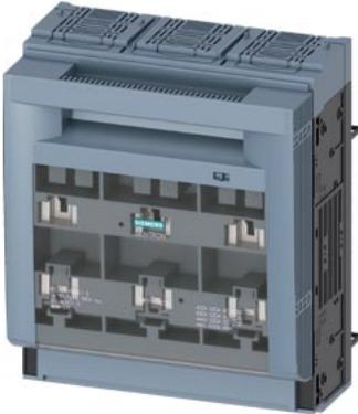
SENTRON, Fuse switch disconnector 3NP1, 3-pole, NH3, 630 A, for Busbar system 8US 60 mm, flat terminal, Cover level 32/70 mm
