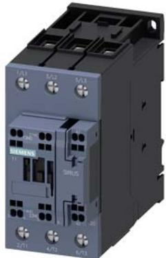
power contactor, AC-3e/AC-3, 65 A, 30 kW / 400 V, 3-pole, 230 V AC, 50/60 Hz, auxiliary contacts: 1 NO + 1 NC, main circuit: screw terminal, control and auxiliary circuit: spring-loaded terminal, size: S2
