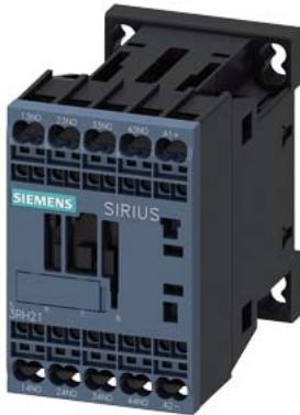
coupling contactor relay, 4 NO, 72 V DC, 0.7-1.25\* Us, with integrated varistor, spring-loaded terminal, frame size S00, suitable for PLC outputs, not expandable with auxiliary switch expandable
