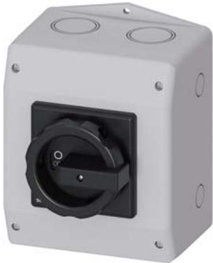
SENTRON, Switch disconnector 3LD, main switch, 6-pole, Iu: 25 A, Operating power / at AC-23 A at 400 V: 9.5 kW, molded-plastic encapsulation for metric cable gland, rotary operating mechanism, black
