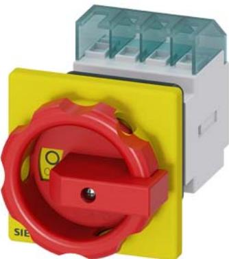
SENTRON, Switch disconnector 3LD, emergency switching-off switch, 3- pole, I<sub>u</sub>: 16 A, operating power / at AC-23 A 400 V: 7.5 kW, front-mounted, rotary operating mechanism, Red / yellow, central mounting 22.5 mm of the handle
