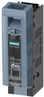
SENTRON, fuse switch disconnector 3NP1, 1-pole, NH000, 160 A, for assembly and installation on mounting plate, box terminal, cover level 45 mm
