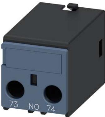
auxiliary switch, on the front, 1 NO, 73/74, current path: 1 NO, cable entry from below, screw terminal, for contactors 3RT2 and contactor relays 3RH2
