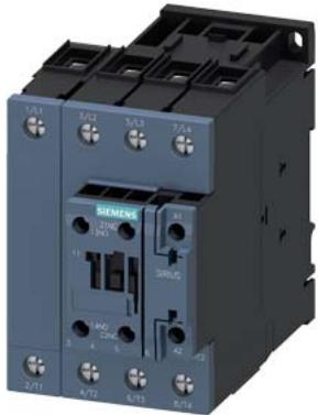
contactor AC-1, 60 A, 400 V / 40 °C, 4-pole, 230 V AC, 50/60 Hz, auxiliary contacts: 1 NO + 1 NC, screw terminal, size: S2
