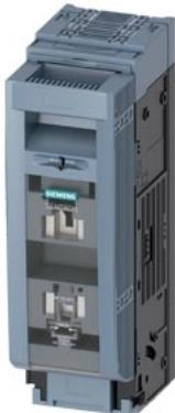
SENTRON, fuse switch disconnector 3NP1, 1-pole, NH3, 630 A, for assembly and installation on mounting plate, Flat terminal, cover level 70mm
