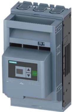
SENTRON, Fuse switch disconnector 3NP1, 3-pole, NH00, 160 A, for assembly and installation on mounting plate, flat terminal, Fuse monitoring: electronic EFM20, Cover level 45 mm
