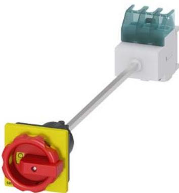
SENTRON, Switch disconnector 3LD, emergency switching-off switch, 3- pole, I<sub>u</sub>: 25 A, operating power / at AC-23 A 400 V: 9.5 kW, floor mounting with door coupling, rotary operating mechanism, Red / yellow, 4-hole mounting of the handle, without tolerance compensation
