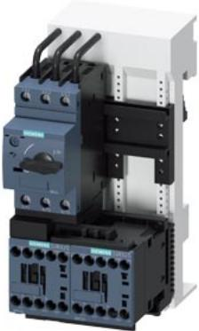
Load feeder fuseless, Reversing duty 400 V AC, Size S00 1.10...1.60 A 24 V DC screw terminal for 60 mm busbar systems (also fulfills type of coordination 1) Type of coordination 2,  $I_q = 150$  kA 1 NC (contactor)
